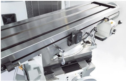
Cutter table swivels in X axis
