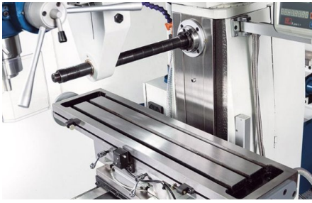
Solid top beam with outer arbor allows rigid mounting of long milling arbors
